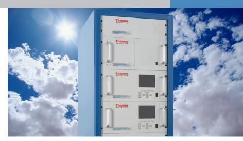
The Thermo Scientific Mercury Freedom System is a complete, integrated solution that includes a probe and internal converter at the stack, plus control, analysis and calibration modules. Data outputs are compatible with existing plant control and data systems. The simple design results in maximum ease of use, lower installation and operating costs, high reliability, easy maintenance and smaller space requirements.
